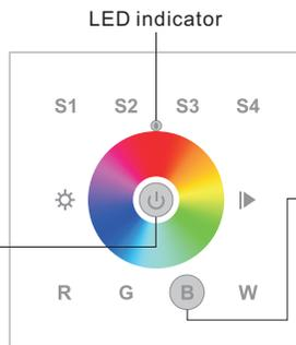
**Step 2:** Short press 5 times continuously to clear all bound lighting devices. LED indicator flashes 4 times for successful unbinding.
