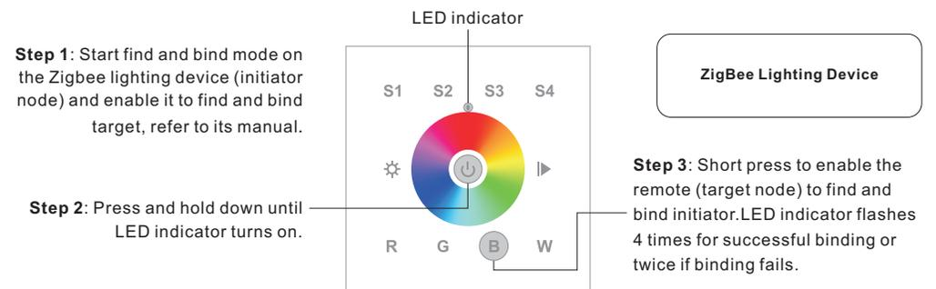
**Note:** Each remote can bind max. 30 lighting devices.
